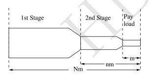
The mass of the second-stage rocket plus the payload, after first-stage burnout and separation, is nm. In each stage the ratio of container mass to initial mass (container plus fuel) is r, and the exhaust speed is V, constant relative to the engine. Note that at the end of each state when the fuel is completely exhausted, the container drops off immediately without affecting the velocity of rocket. Ignore gravity.
