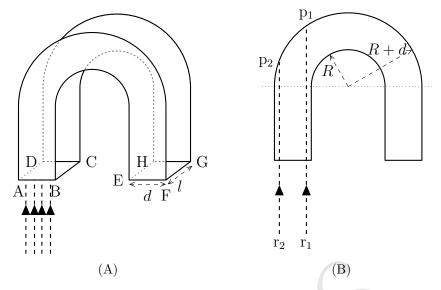
Bent portion of the rod is semi-circular with inner and outer radii R and R + d respectively. Parallel monochromatic beam of light is incident normally on face ABCD.
