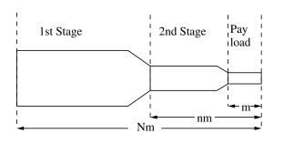
The mass of the second-stage rocket plus the payload, after first-stage burnout and separation, is nm. In each stage the ratio of container mass to initial mass (container plus fuel) is r, and the exhaust speed is V, constant relative to the engine. Note that at the end of each state when the fuel is completely exhausted, the container drops off immediately without affecting the velocity of rocket. Ignore gravity.
